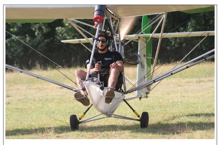
The mylar hull emphasizes the line of the fuselage and the front skid
